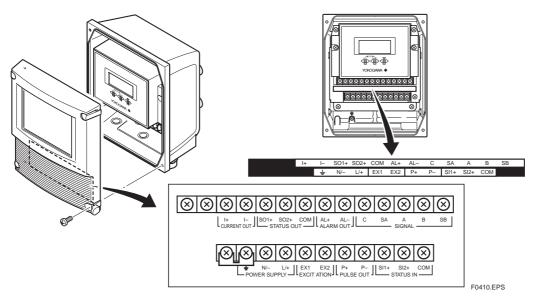
Figure 4.4.2 Terminal Layout Labels Position
